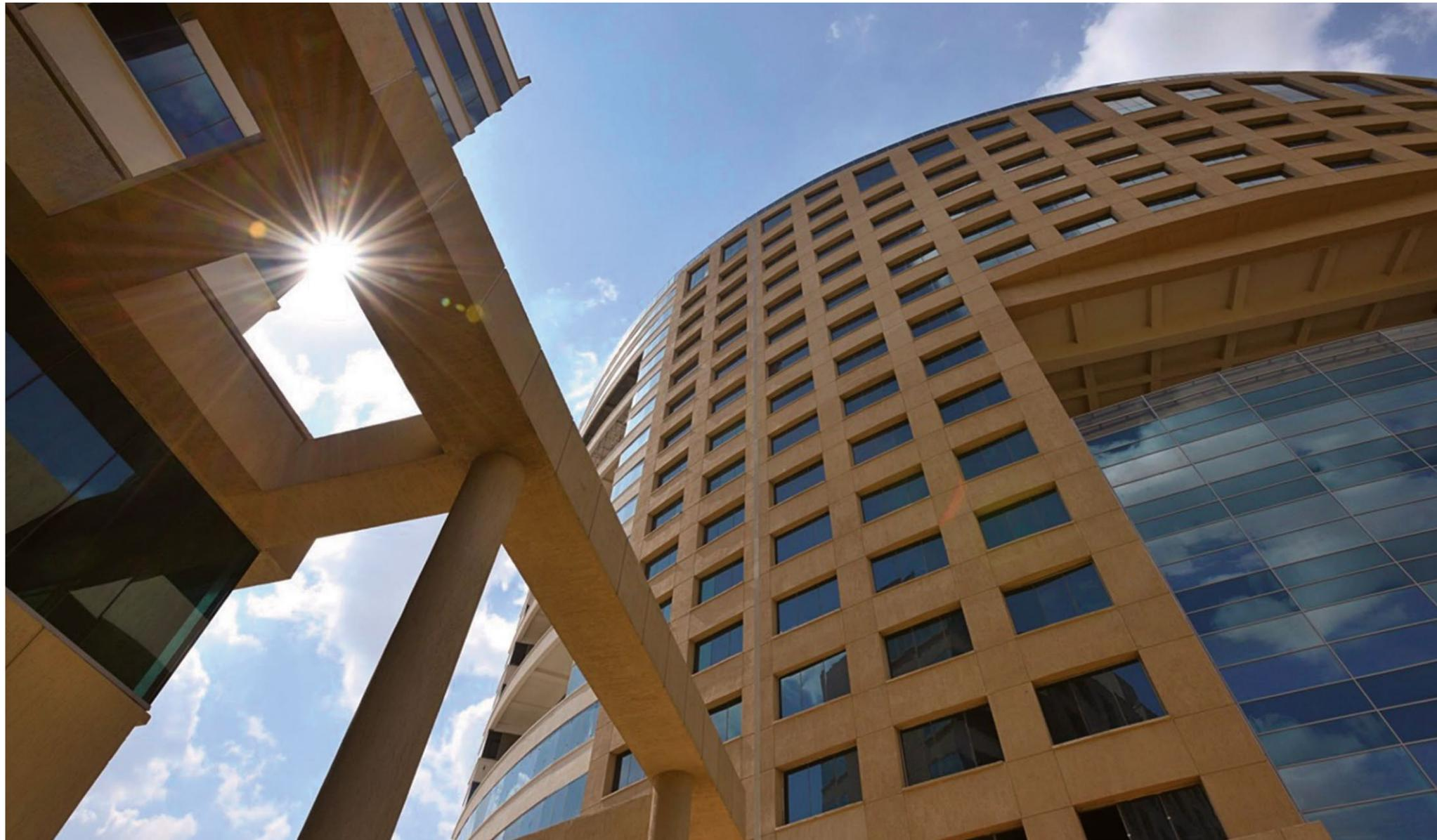
Cyberwalk has a dedicated area of 25,000 sq-ft to 38,000 sq-ft for commercial office space. Since the building aimed at a LEED rating, the architect selected SGG Envision glass, a high performance material with excellent thermal insulation properties and high spectral selectivity. In addition to delivering a superior performance, Envision also enables abundant light transmission and is relatively more transparent than other solar control glasses.
