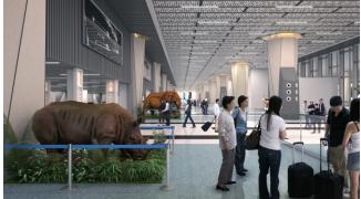
Claim hall wall is an exercise in modularity with Origami aluminum panels that derive inspiration from the hilly terrain of the North-eastern states.
